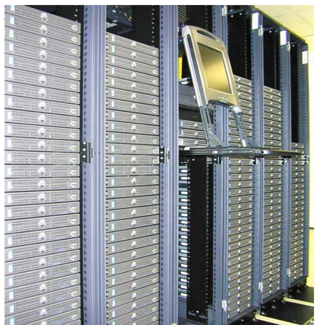
ac3's new Dell Cluster computer, "Barossa", comprises 155 dual processor nodes, providing a sustained computing power of over a teraflop.
