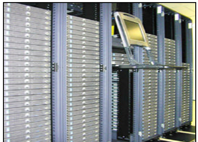
ac3's Dell Linux Cluster has been upgraded with an additional 32 dual processor nodes to bring the total number of nodes to 187.
