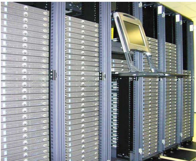
ac3 's 310 processor Dell Linux cluster supercomputer established a world record for Oracle. 120 of its processors were used as a database server to access a single database.
